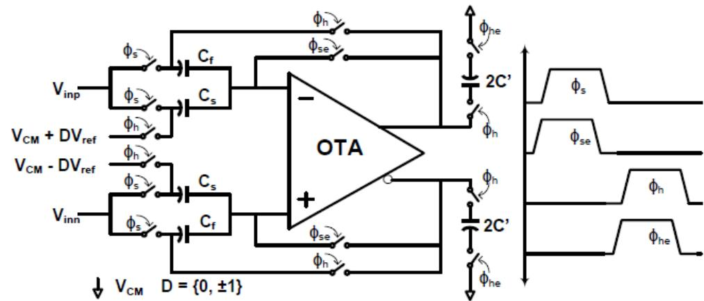
MDAC block diagram (subADC not shown here)
