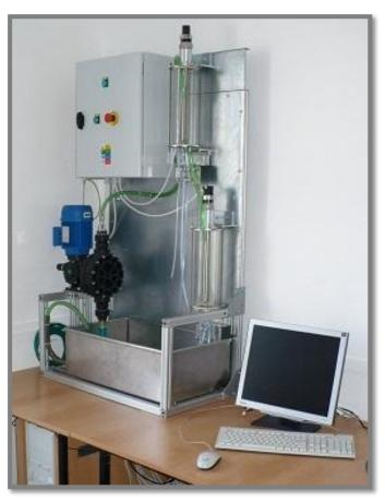
Hydraulic system with frequency converter
