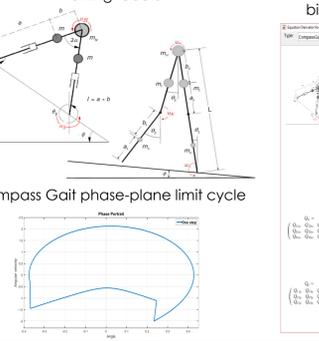
Automatic generation of continuous and discrete dynamics (motion and transition equations) for passive bipeds with optional knees, torso and feet
