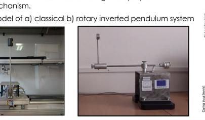
Swing-up and LQR stabilization of a classical single inverted pendulum with a linear synchronous motor
