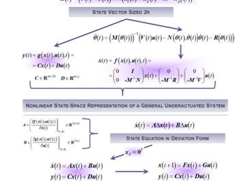
Linear approximation of classical and rotary inverted pendulum systems around a given equilibrium point
