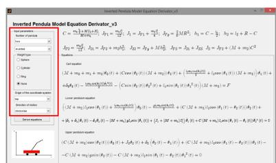
Automatic generation of motion equations for an Acrobot, Pendubot and Inertia Wheel Pendulum with optional reference link position
