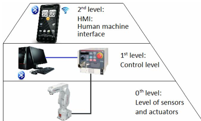
Fig. 1: Hierarchic architecture of described system.
