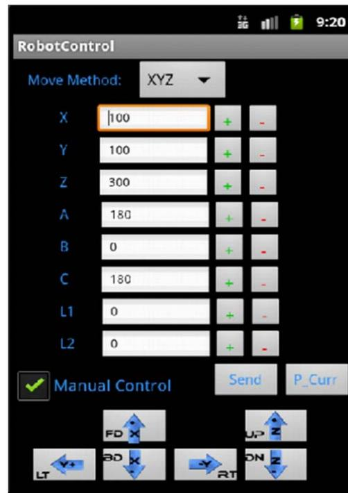
Fig. 7: RobotControl Activit (SP screen).
