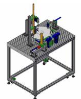
Fig. 7. Graphic design of the Post 4- Inserting plastic shaft and metal hats.
