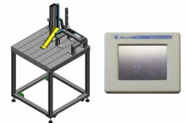
Fig. 6. Graphic design of the Post 3 – Inserting bearings rack (A). PanelView Plus 600 (B).
