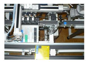
Fig. 6 Colour monitoring sensor with device to sort out cubes
