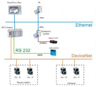
Fig. 5 FMS devices interconnection
