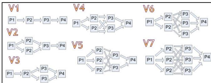
Fig. 3 Possible alternatives of assembly line configuration
