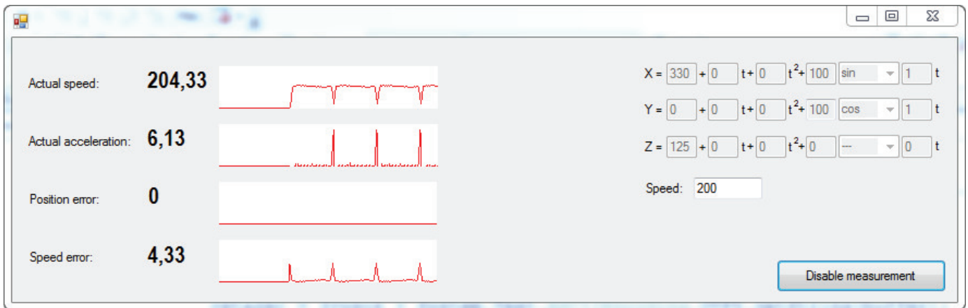
Fig. 1. Diagnostic tool for movement of industrial robot MELFA RV-2SDB
