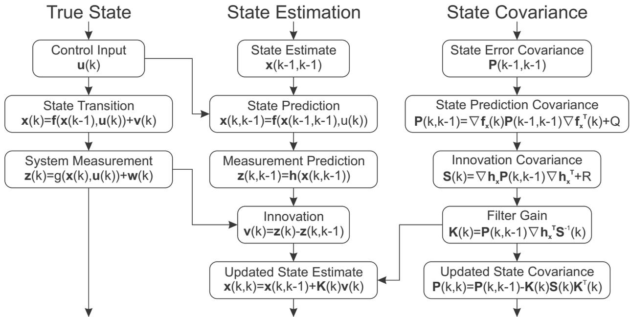
Fig. 1: Block diagram of the Extended Kalman filter cycle [8], [18]
