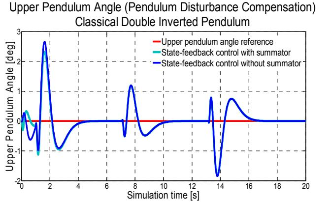
Figure 12. Classical double inverted pendulum: simulation results for LQR control with a summator – upper pendulum angle
