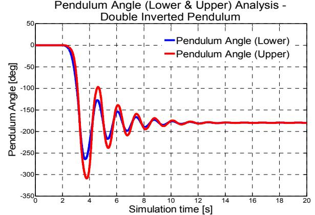
Figure 4. Classical double inverted pendulum (*force model*) – open-loop time behavior of pendula angles
