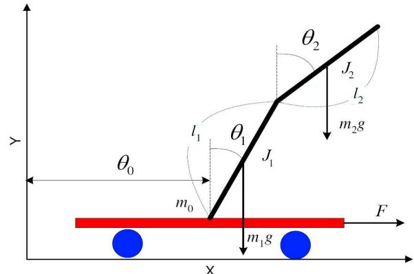
Figure 1. Classical double inverted pendulum system – scheme [4]
