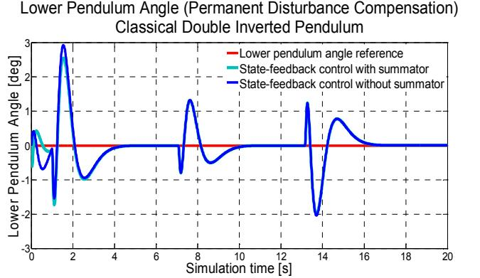
Figure 11. Classical double inverted pendulum: simulation results for LQR control with a summator – lower pendulum angle
