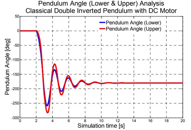
Figure 6. Classical double inverted pendulum (*voltage model*) – open-loop time behavior of pendula angles
