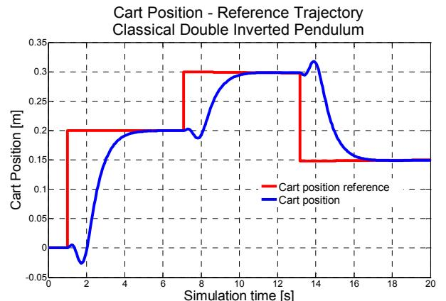
Figure 8. Classical double inverted pendulum: simulation results for pole-placement control – cart position
