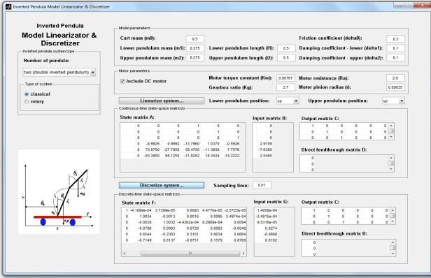
Figure 7. Obtaining the linearized and discretized state-space matrices in the upright position of the classical double inverted pendulum voltage model using the *Inverted Pendula Model Linearizer & Discretizer*
