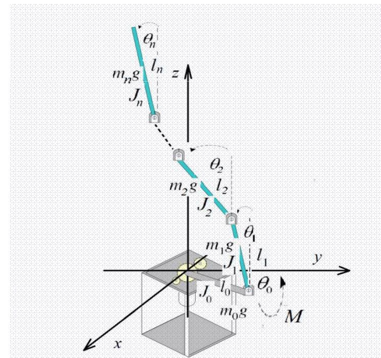
system of  $n$  rotary inverted pendula
