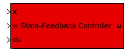
State-Feedback Controller with Feedforward Gain
