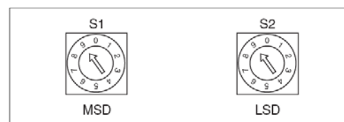
Fig. 4. Setting addresses of motors
