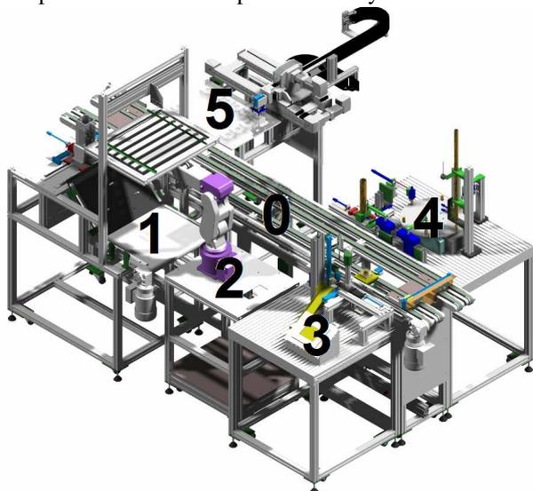
Fig. 3. Graphic design of the assembly line with the numbered posts.
