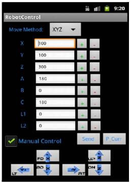
Fig. 7: RobotControl Activit (SP screen).
