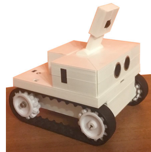
Fig. 10. Fully assembled prototype with sensor modules
