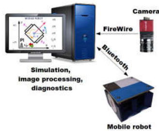
Figure 4. Laboratory workplace for the mobile robot control and diagnostics – conceptual scheme
