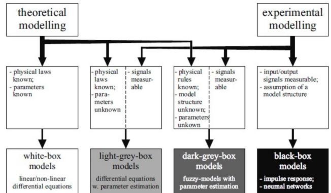
Fig. 2 Different kind of the nonlinear systems models [17]
