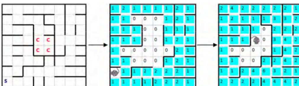
Fig. 2 Maze solving using improved right hand method.
