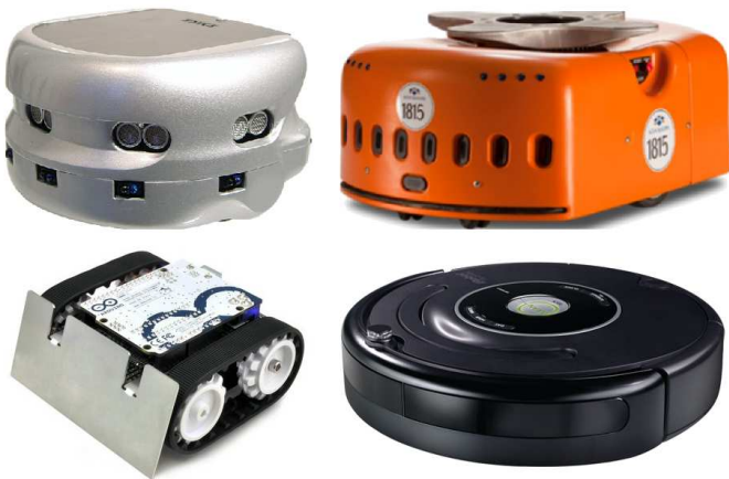
Fig. 1. Example of commercially available mobile robots with differential drive (Khepera III, Kiva, Zumo, Roomba).
