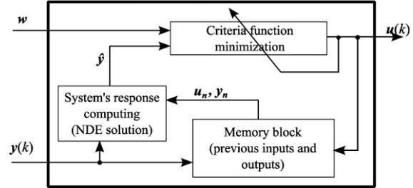
Fig. 2 Nonlinear predictive control algorithm
