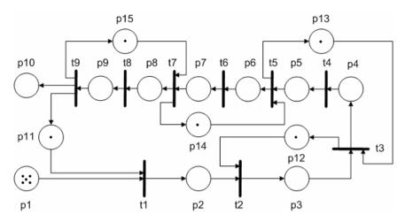
Fig. 2. Petri net modeling the flexible production system
